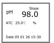
If you would like to know electrode's slope value after pH calibration, press [Slope] key. The slope value is displayed in the main field of screen and disappeared.
