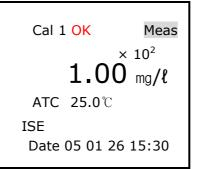
Right one is indicated of finishing of the first buffer's calibration
