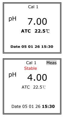
From pH ready, press [Cal] Key to move Cal 1 then left display is shown.
