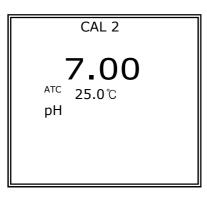
2) Calibration of CAL2.to CAL3 (Buffer2 to Buffer3) Calibration method of Cal2 to cal3 is same with cal 1. When you finished 3points, it is exit to pH initial display. Rinse the sensor with distilled water and put it into the Second Buffer for next calibration.
