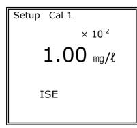
From ISE Ready Mode, press [Setup] key to enter in left display. And press [Select] key to find proper standard solution  $1.00 \times 10^{-2}$ ,  $1.00 \times 10^{0}$ ,  $1.00 \times 10^{1}$ ,  $1.00 \times 10^{2}$ ,  $1.00 \times 10^{3}$ . And press [Memory] key to selecting standard solution what is displayed.
