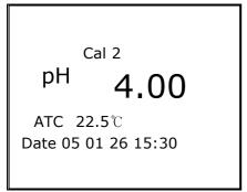
Calibration method of Cal2 to Cal 5 is same with cal 1.(For pH-200L, maximum is Cal 3 ,But pH-220, pH-240 it can be calibrated until 5 points maximum)
