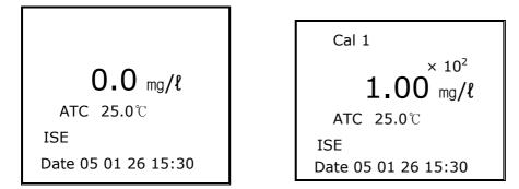
At first, rinse the sensor with distilled water carefully, remove moisture clearly and put in the electrode into first calibration Buffer<Cal 1> and stir it carefully for a while and press [Meas] Key, then Meas is appeared on the screen and Calibration buffer's ION vale is also indicated.
